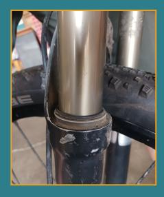
With weight over handlebars, 'bounce' to activate forks, then let settle. Move O-ring against dust wiper. Dismount carefully!
