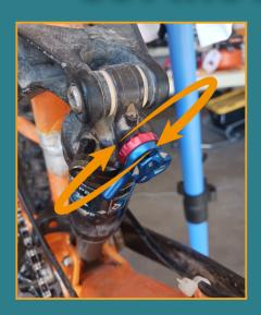
Set the shock rebound dial to full damping (+)/ all the way clockwise. Then follow the same procedure as step 08, OR continue to step 11.
