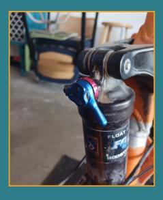
The middle setting is usually a good base setting for most riding. Switch to full damping when climbing, less damping for gnar downhills.
