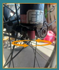
Move dial 2 clicks counterclockwise (-) to decrease damping and repeat step 08 until rebound is fastest w/o tire lifting off the ground.
