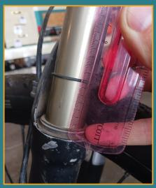
The distance between 0- 06 ring and dust wiper is the sag. Measure and add or release air to achieve 25% sag. Repeat step 05 & 06.
