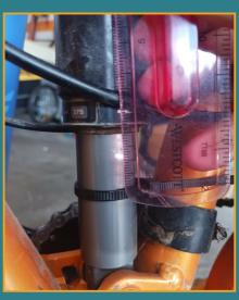
The distance between O- oring and dust wiper is the sag. Measure and add or release air to achieve 25% sag. Repeat steps 03 & 04.
