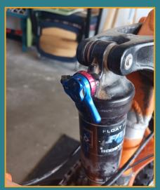
Eliminate any compression damping by turning compression dial/lever (blue) all the way counter-clockwise (-)
