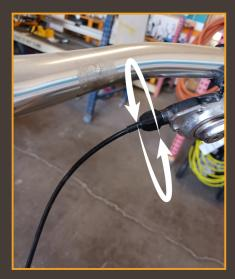
Turn barrel adjuster 05 counter-clockwise until you begin to hear excessive chain noise (of chain wanting to shift one lower).
