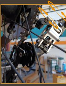
Turn B-Limit screw clockwise to increase the distance; turn counter-clockwise to decrease distance.
