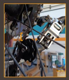
In easiest gear, note distance between largest cog and guide pulley.
