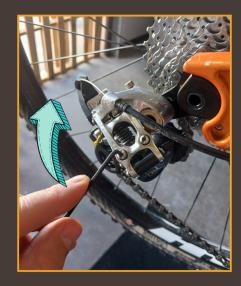
Turn H-Limit screw C2 clockwise until there is noise from the chain (wanting to shift one cog easier)
