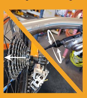
...turning barrel adjuster counter-clockwise...
