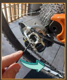
Turn H-Limit screw C3 counter-clockwise in very small increments until noise ceases
