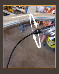
Now turn barrel adjuster 06 clockwise in small increments (¼ turns) just until excessive chain noise is eliminated.
