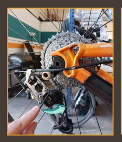
Now turn L-Limit screw counter-clockwise in smaller increments until excessive noise is eliminated and it shifts to easiest gear easily.
