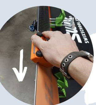
With ski secured in top of guide blocks draw tuner over base edge with short, overlapping pulls. Then one long pull.
