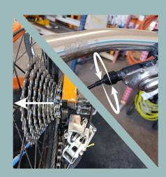
The barrel adjuster is a bit counter-intuitive. Loosening the adjuster will lengthen the cable housing which will tighten the cable. Soooo...
