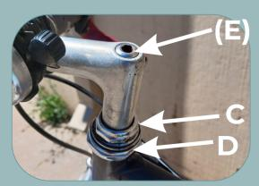
For loose <u>threaded headsets</u>: Loosen locknut (C) while securing race (D) in place, finger tighten race (D), then tighten locknut (C). The stem bolt (E) adjusts stem height/alignment.
